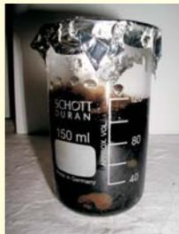
Sample after treatment by a centrifuge. Only a small amount of water was separated.
