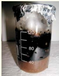
Sample after treatment by the special ESSORP-Ultrasonic-Technology. The complete emulsified water was separated from the oil.
